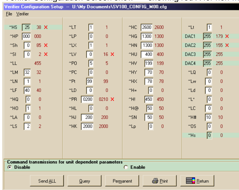
Figure 5 – Verifier Configuration Screen show -- showing red X for non-match Query
